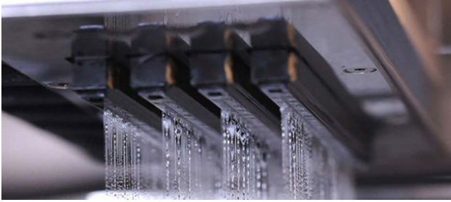
Figure 5. Printhead jetting furfural alcohol-based binder.
