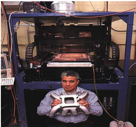
Figure 2. DSPC, Soligen Technologies Inc.'s Beta generation machine, and CEO and creative Yehoram Uziel.
