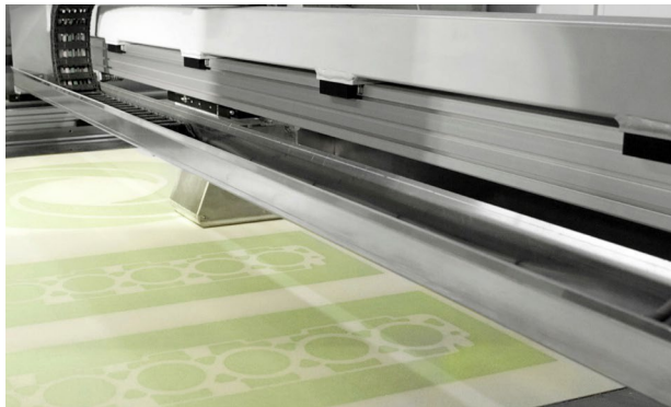
Figure 6. Printed bed with cured furfuryl-alcohol printed cores and activator-coated but unprinted sand.
