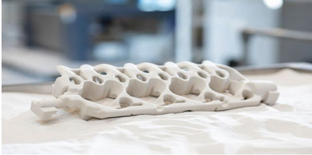
Figure 9. A complex core 3D printed with inorganic binder and silica sand. (Artwork courtesy of ExOne.)
